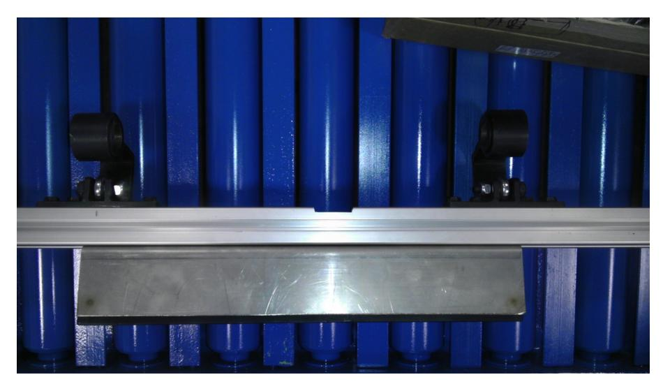
4 – New Back Stop Assemblies Labeled for each pocket Pockets 1 &2 – Assembled with 10 lb Springs (Part 094746) Pockets 3 & 4 – Assembled with 5.5 lb Springs (Part 259017) A 4 lb spring in included. All springs are interchangeable.
