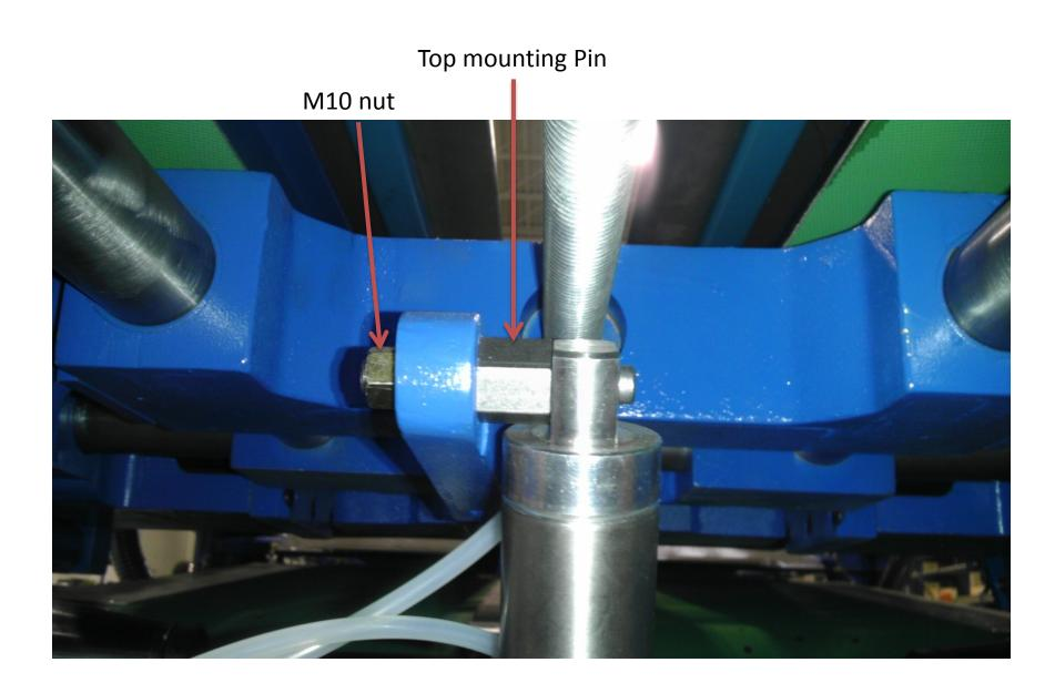
Remove Back Plate Support and Pad. Remove 3 - M10 screws, lock washers, and support pins from each side. Save Bolts, Washers, and Support Pins
