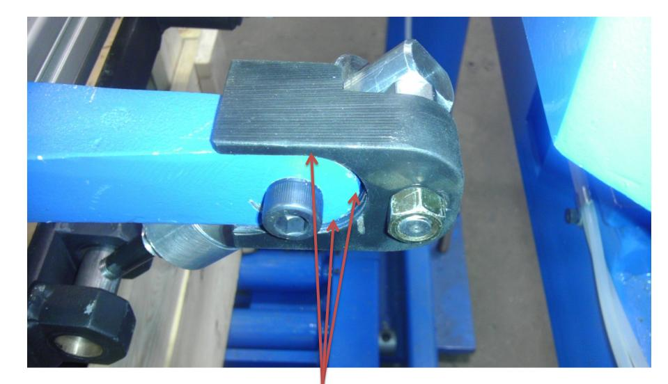
Some grinding of the casting may be required in order to fit the cylinder adapter.
