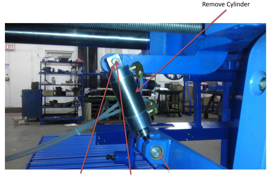
Save Hardware - Retaining Clip Top Mounting Pin Shaft & M10 Nut
