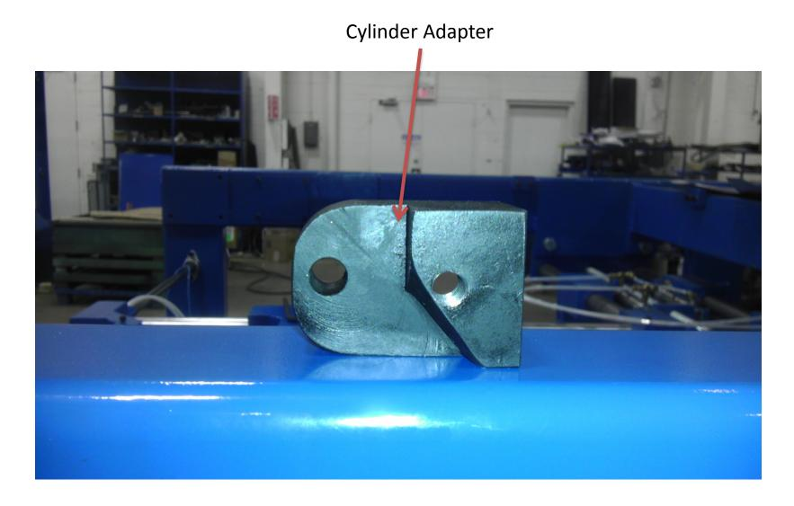
Attach Cylinder with mounting pin & retaining clip saved from Cylinder Removal. Attach Cylinder Adapted with included M10 Bolt
