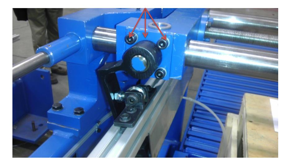
There may be a gap between the new back stop assembly support and the support pin. Install one of the included washers. 1.00 ID x 1.50 OD x .12 thick.
